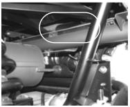
NOTICE: Water in the PVT system could cause the drive belt to become wet and slip in the clutches. Always avoid spraying water directly toward the PVT outlet duct when washing the vehicle from the rear.
